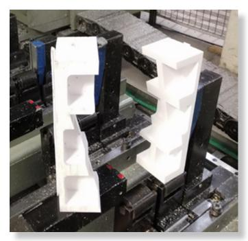
They tried using plastic on a CNC mill, however, while that technique was fast, it required significant expertise. With Rize One, NHF produces accurate, low cost clamping fixtures at \$50 per part. This amounts to a savings of up to \$50K per quarter on the clamping fixtures alone.
