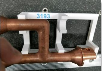
HMS also uses Rize One's breakthrough 3D printed marking capability, made possible with Rize's voxel-level Augmented Deposition process, to indicate, right on the part, the location where the part should be placed and part numbers for identification.
