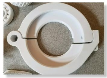
With their Rize One 3D printer, HMS employees design and print parts on demand in one day, freeing up a team member and saving up to two days per fixture vs. producing aluminum fixtures, and only costing approximately \$40.00 per part.
