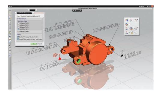
Siemens provides a comprehensive 3D annotation environment that not only captures and associates manufacturing requirements to the 3D model, but also allows the digital data to be re-used by downstream applications because the data lives with – and is driven by – the product's parts.
